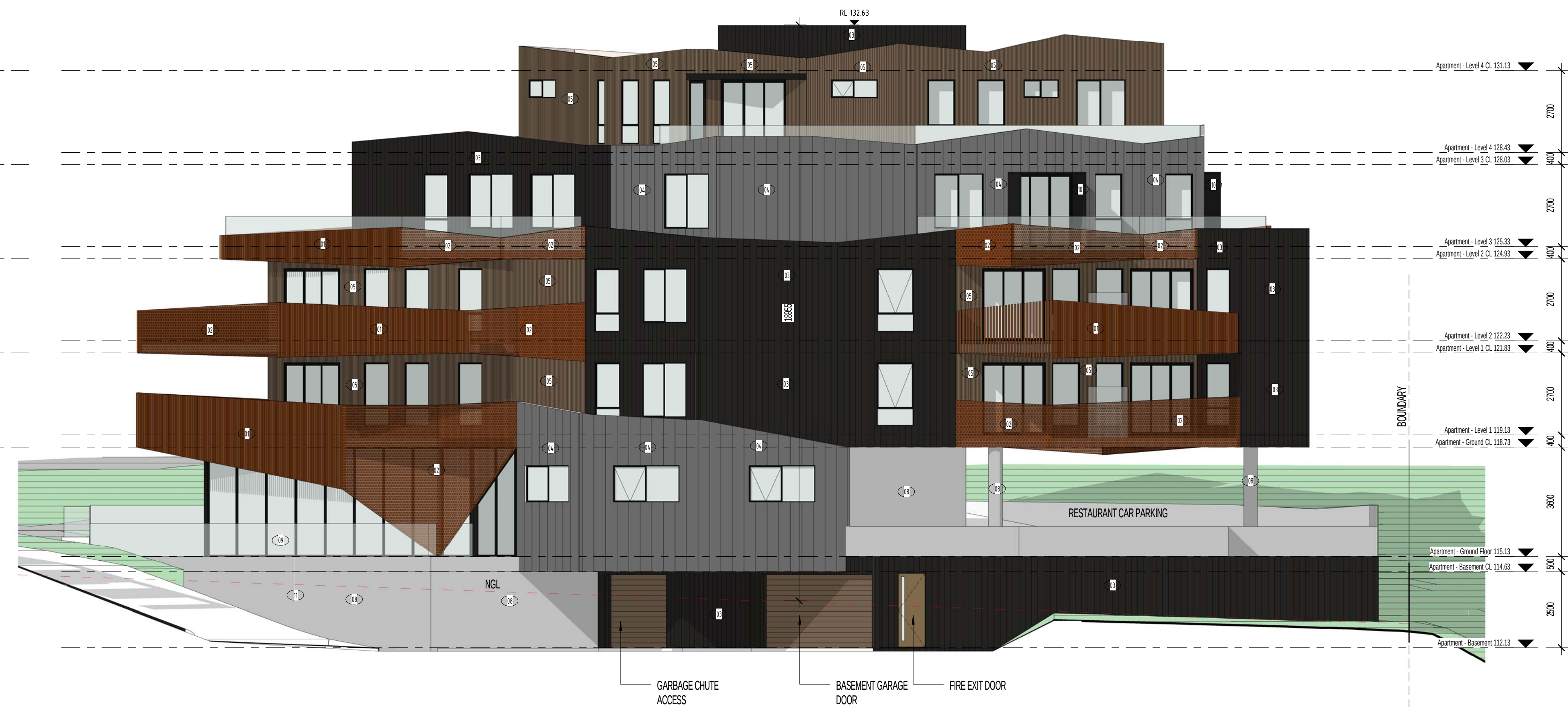
2 Apartment - North Elevation 1 : 100
